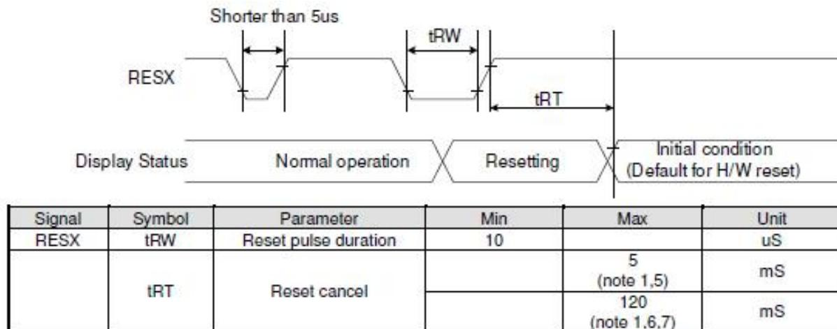
*Note 1: The reset cancel includes also required time for loading ID bytes, VCOM setting and other settings from NV memory to registers. This loading is done every time when there is HW reset cancel time ( $t_{RT}$ ) within 5 ms after a rising edge of RESX.*
