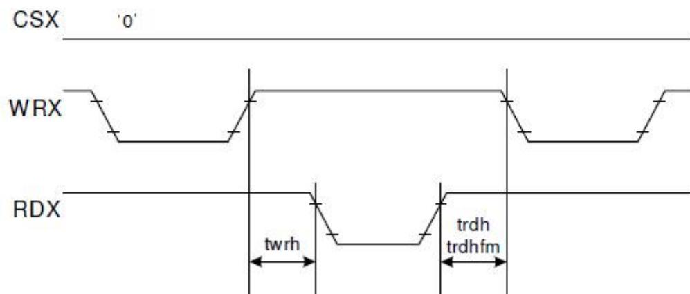
Note: Logic high and low levels are specified as 30% and 70% of IOVCC for Input signals.
